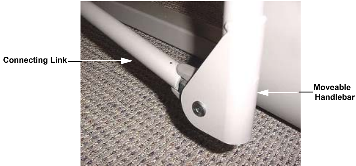
Diagram 7.14 - Moveable Handlebar, Lower End
