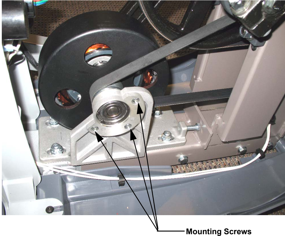
Diagram 7.8 - Generator Mounting, Pulley Side
