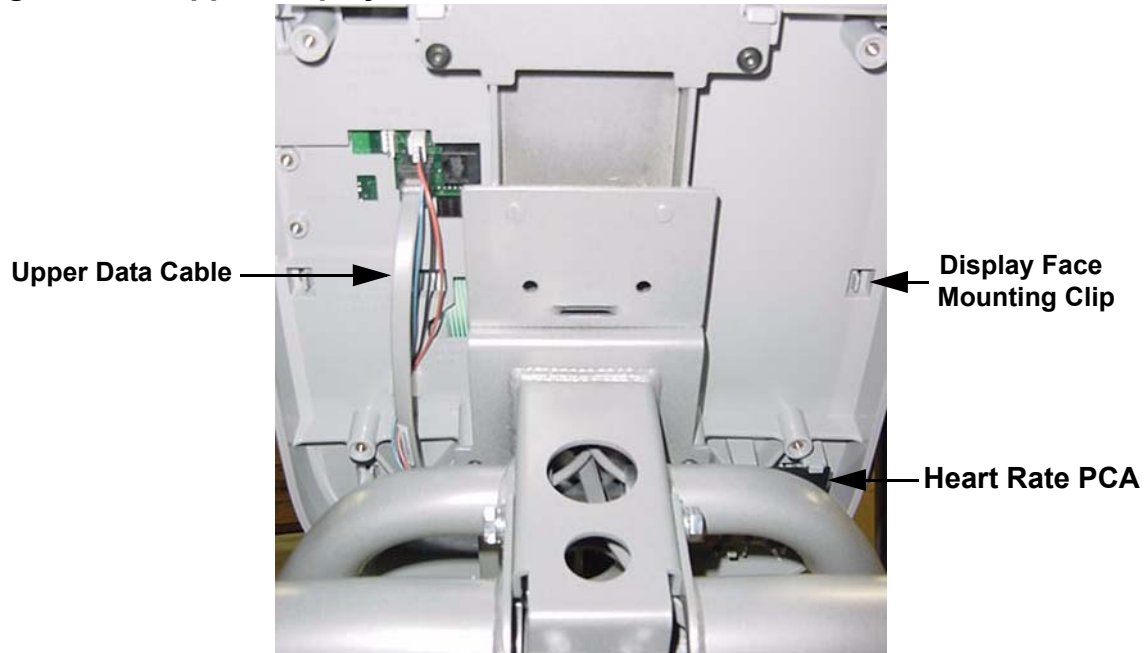
Diagram 6.2 - Upper Display Cable
